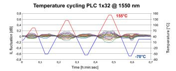
Survived 100x cycles of temperature shocks between -70°C and 155°C.
